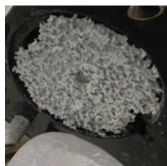
Unprotected and premature transom & outdrive zinc loss
